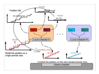
Fig. 1. Compositional system model.
